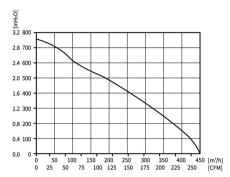
Motor Type Wiring Mode Speed Control Protection Type Insulation Class Operating Temperature Weight DC BRUSHLESS EXTERNAL ROTOR MOTOR IP55 1.2KG D1 -25°C~+60°C
