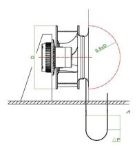
The differential pressure approach compares the static pressure before the inlet nozzle with the static pressure inside the inlet nozzle. Air flow can be calculated on the basis of the differential pressure (difference in pressure of the static pressures) in keeping with the following equation:
